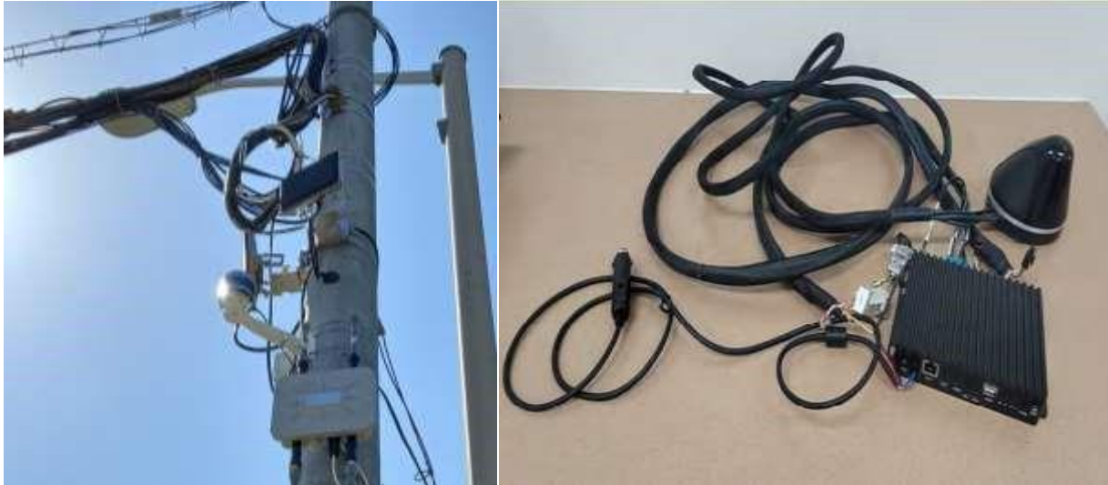
Figure 2 LiDAR Sensor, RSU, and OBU Setup on the Morgan State University CAV Testbed Figure 3 shows the CCTV cameras installed at both intersections on the CAV testbed.
